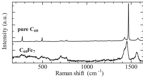
Fig. 1. Raman spectrum of the  $C_{60}Fe_7$  film and that of a pure  $C_{60}$  film for comparison.
