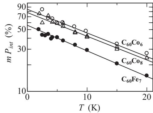
**Fig. 6.** Interface spin polarization ( $P_{\text{int}}$ ) multiplied by the relative magnetization ( $m \leq 1$ ) of the Fe nanoparticles involved in the transport plotted as a function of temperature. The solid circles, open circles and open triangles represent the data for  $C_{60}Fe_7$  (present sample),  $C_{60}Co_6$  and  $C_{60}Co_8$  (Refs. [11,12]), respectively. The solid lines represent the best-fits to Eq. (2) for the respective samples.
