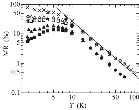
**Fig. 5.** Plot of the MR ratios at  $H=10$  kOe (solid symbols) and 70 kOe (open symbols) measured under  $V=20$  V (circles), 60 V (triangles) and 80 V (squares) and the zero-bias MR ratio at  $H=70$  kOe (crosses). The measurements were not made in the range of  $T < 8$  K at  $V=20$  V and in the range of  $T > 10$  K at  $V=80$  V because of the high resistance and the temperature-rise of the device under these conditions.
