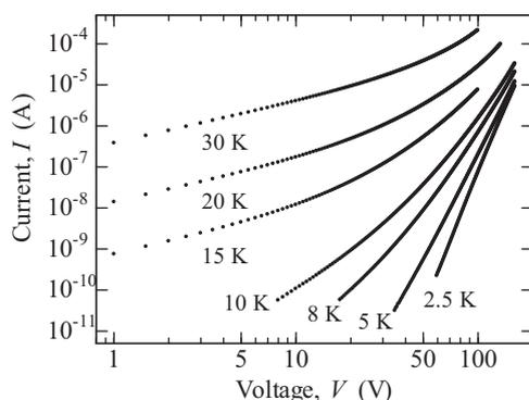
Fig. 2. Current-voltage characteristics of the 100-nm-thick  $C_{60}Fe_7$  film measured under the CIP geometry at different temperatures.
