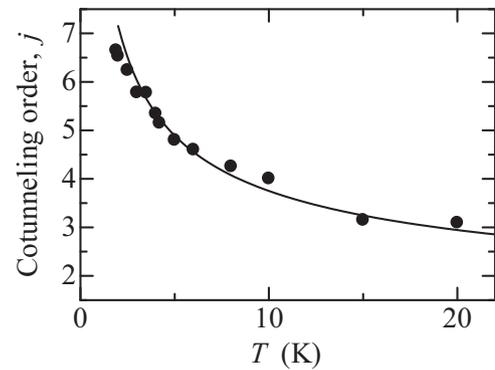
Fig. 3. Cotunneling order  $j$  as a function of temperature. The solid line represents the fit with the theoretically proposed dependence for granular systems (see text for details).
